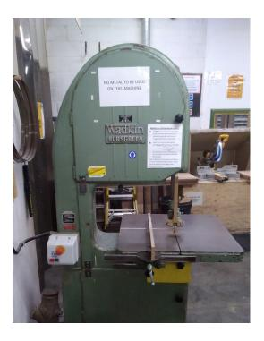
Bandsaws are generally lower risk machines than circular saws and are used for cutting curves or thicker sections of timber than other saws can manage. Their thin blade also produces less waste than other types of saw.
