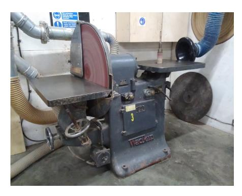
Machine sanders are generally more accurate than sanding with power tools. It is also easier to connect them to a proper dust extraction system, and so are preferable to use for sanding in a workshop environment. Sanding machines are available in different forms, depending upon the task to be carried out. These are defined below:
