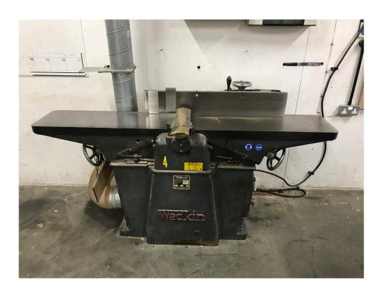
The Surface Planer and Thicknesser are used to plane accurate smooth surfaces on four sides of your timber. You are likely to need to do this when you have purchased 'sawn' timber from a supplier, or simply need to reduce pre-planed timber or board materials down to your required measurements.
