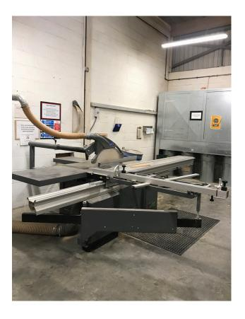
Table-saws are in principle a basic machine, comprising a circular saw blade which protrudes up through a slot in the centre of a flat worktable. This is turned by a powerful motor and drive system, which is mounted beneath the machine. Fitted with fences and guards, the machine is used to cut down solid timber and board materials to size. Table saws are also known as panel saws, dimension saws, rip saws and mobile site sawbenches and vary in design and size depending upon their intended use.
