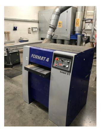
The Thicknesser is used to plane accurate smooth surfaces on the remaining two faces of your timber (opposite the face side and edge previously machined on the surface planer). It is also useful for reducing the thickness of material that is already machined and for flattening wider surfaces on boards made from two or more glued-up components – e.g. solid table tops.
