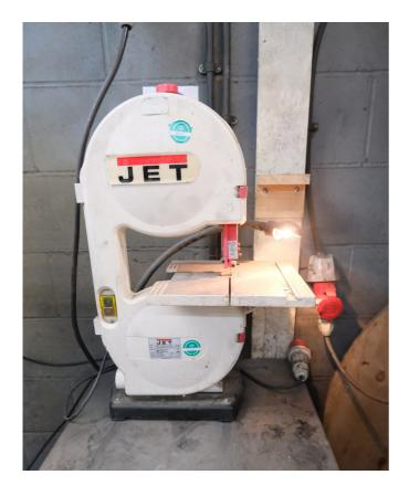
The Bandsaw is used for detail cutting of thin sheet material only. It's blade is suitable for non-ferrous materials only (i.e. brass, copper and aluminium) and can cut up to a thickness of 2mm.
