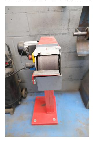
The Belt Linisher is commonly used for grinding and preparing the surface of metals. It has a flat sanding belt which can be used to flatten surfaces or remove the 'burrs' or sharp edges of etn left after cutting on the coldsaw.
