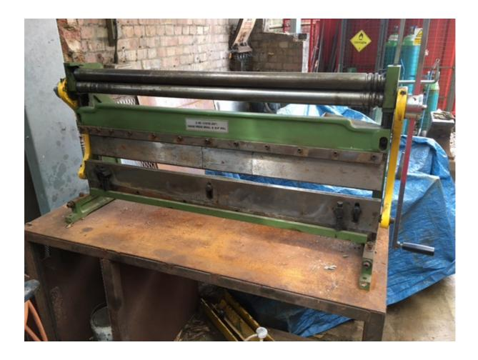
The smallest diameter of roll that can be achieved is 42mm, with the top roller being removable to allow the workpeice to be removed from the machine. Grooves on the right-hand end of the rollers also allow the bending of 6mm, 8mm and 10mm solid round bar.
