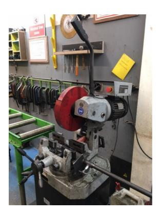
The cold saw is a powerful motor-driven machine used for cutting down metal lengths as large as 150 x 100mm in section. The machine has a hardened blade which is capable of cutting through most metals.the machine is fitted with a pump-fed coolant system to prevent damage to the blade, which activates when the motor is started by the switch on the handle. For safety, the blade is guarded and the workpiece is held securely in a vice while the material is being cut.
