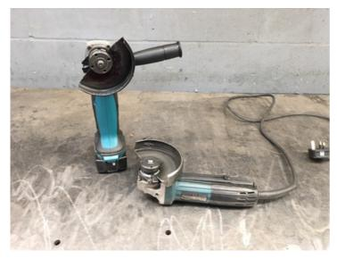
The angle grinder is one of the most commonly used in metalwork, and is used for cutting and trimming metal, dressing down welds and prepairing joints prior to welding. Despite it's small size, there are numerous risks of injury when using an angle grinder, and so it is essential to ensure you are using it safely at all times.
