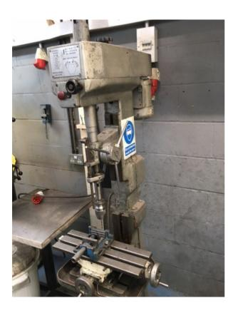
Pillar Drills (or drill presses) provide a more accurate and safer means of drilling holes than a hend-held drill. They are also more powerful and so better suited to drilling larger diameter holes. Workpeices can easily be clamped to their adjustble bed or held in a vice, allowing for greater control over the drilling process.
