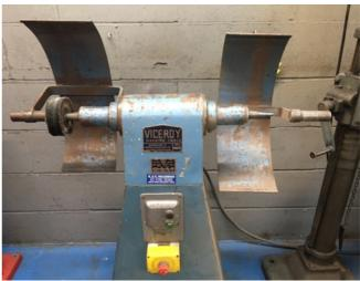
These are used for sharpening of tools and cleaning/polishing of metal surfaces. The bench grinder is fitted with an abrasive wheel which is used for sharpening hardened tools such a drill bits and lathe tools, as well as precision grinding of tube joints for brazing or welding. The bench grinder also has a wire wheel which is used for removal of paints and rust from surfaces, as well as cleaning of bolt threads ect.
